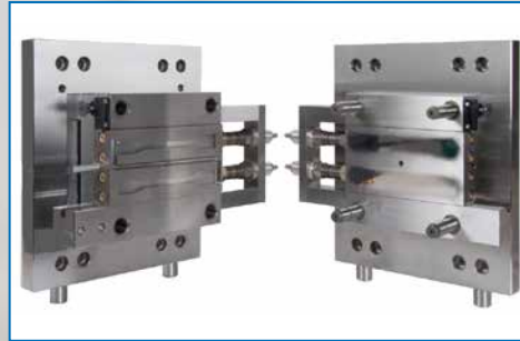
Master tool with interchangeable insert and mirror plate
