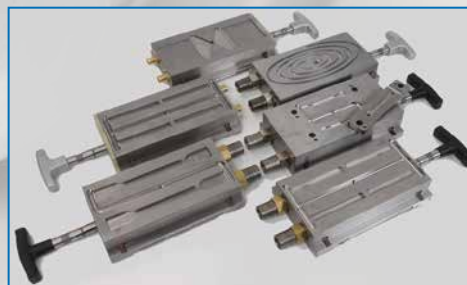
moving mould half side inserts
